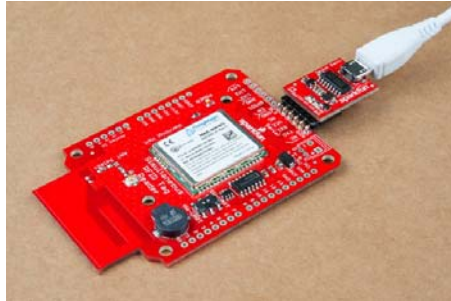
USB power only. Limited to 5dBm read power.
