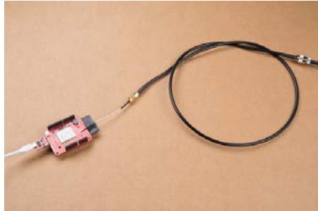
u.FL connector to RP-SMA to RP-TNC
