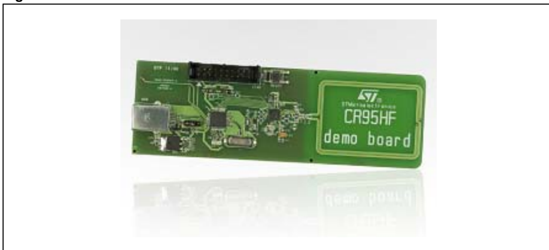
Figure 15. DEMO-CR95HF-A demonstration kit
