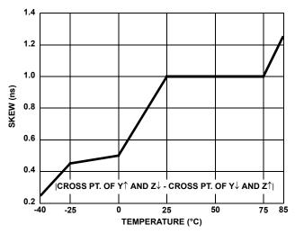
FIGURE 14. DRIVER DIFFERENTIAL SKEW vs TEMPERATURE (ISL83073E, ISL83075E)
