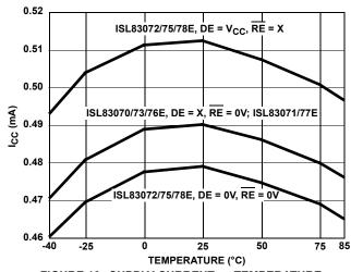
FIGURE 10. SUPPLY CURRENT vs TEMPERATURE
