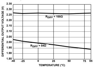
FIGURE 8. DRIVER DIFFERENTIAL OUTPUT VOLTAGE vs TEMPERATURE
